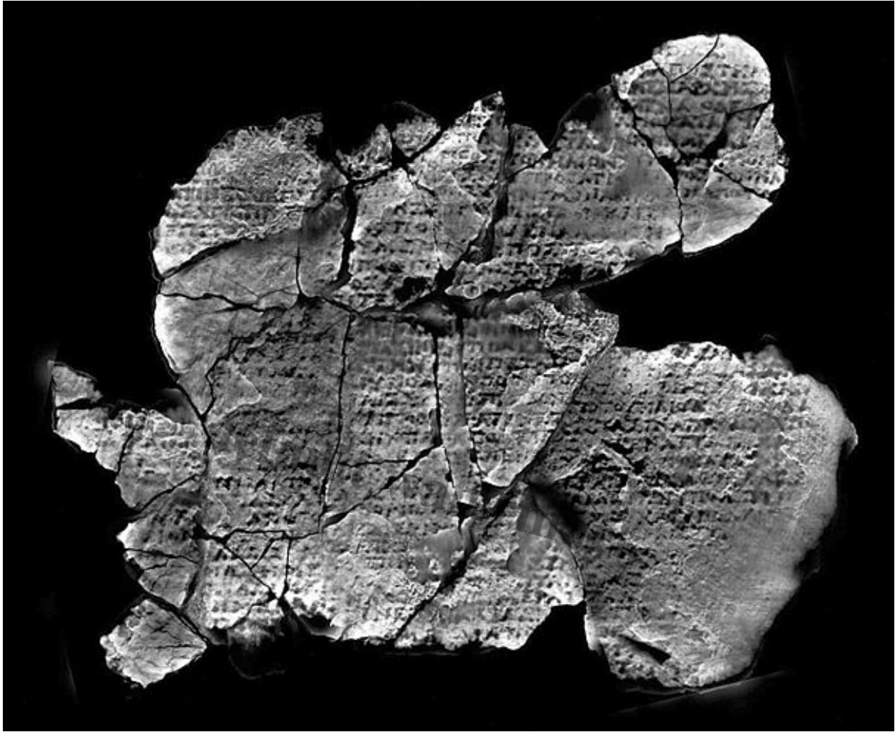
Hidden message: X-ray CT scans made in 2005 revealed previously unseen inscriptions on the Antikythera mechanism, including a list of planetary cycles on the front cover ( shown here ) and a “user’s manual” on the back cover. Credit: © 2005 Nikon X-Tek Systems
